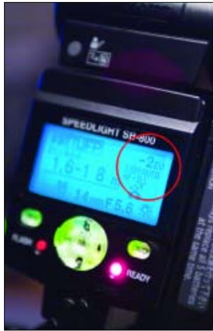
Left—Example of off-camera flash and a dedicated sync lead. Right—EV flash compensation set on the flash unit at -2.0 stops.
